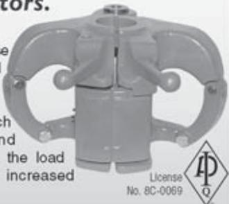
Now called PETOL "BIG D" these tubing elevators are constructed of high-quality alloy steel and heat-treated for maximum strength and durability. Each elevator is manufactured and tested to API 8C. In addition, the load collar is flame hardened for increased abrasion resistance.
